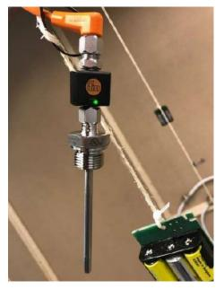
$\leftarrow$  In the centre of the test-room a temperature sensor was installed, acting as the room thermostat
